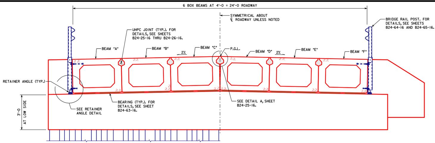
**SECTION NEAR ABUTMENT WITH SHEET PILE WINGS**
