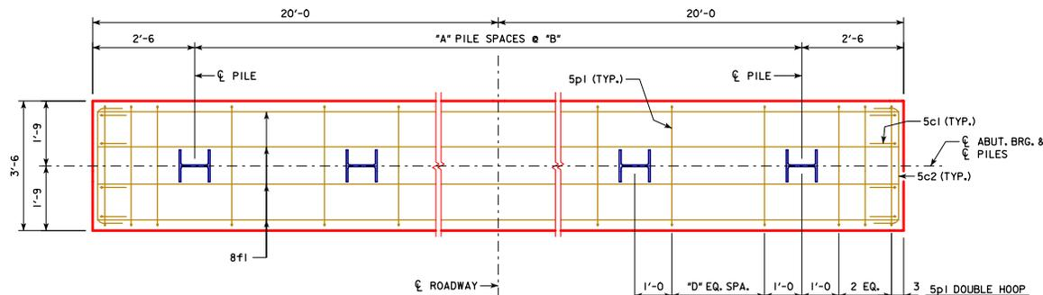
ABUTMENT PILE PLAN
