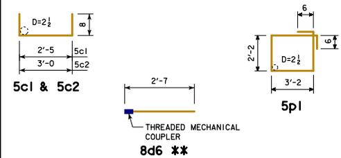
NOTE: ALL DIMENSIONS ARE OUT TO OUT. D= PIN DIAMETER.
