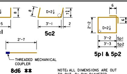
NOTE: ALL DIMENSIONS ARE OUT TO OUT. D= PIN DIAMETER.
