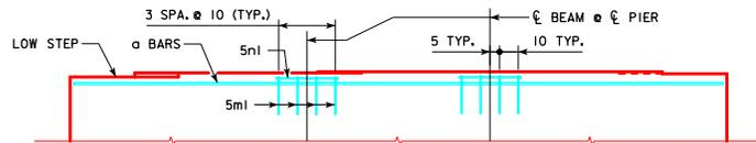
**PART ELEVATION VIEW OF PIER CAP**
