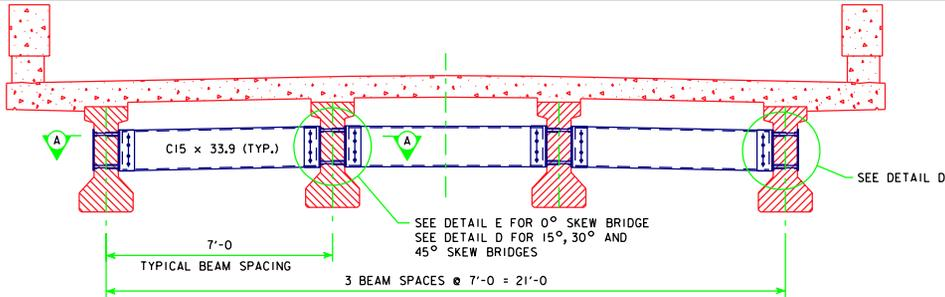
SECTION SHOWING INTERMEDIATE DIAPHRAGM
