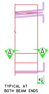
**STRAND PROJECTION AT BEAM ENDS WHEN EMBEDDED IN CONCRETE END DIAPHRAGMS**
