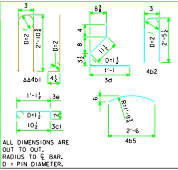
ALL DIMENSIONS ARE OUT TO OUT. RADIUS TO  $\phi$  BAR. D = PIN DIAMETER.
