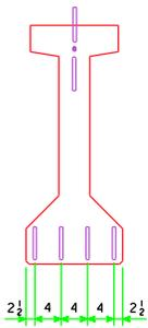
2 TOP DEFLECTED OR STRAIGHT STRANDS ARE TO BE CUT WITH 1'-0" PROJECTIONS AND SHOP BENT UP OR DOWN AS SHOWN (BEND TOP AND BOTTOM ROWS). THE REMAINING TOP STRANDS ARE TO BE CUT WITH 0'-3" PROJECTIONS. FOUR BOTTOM STRANDS ARE TO BE CUT WITH 1'-0" PROJECTIONS AND SHOP BENT AS SHOWN. THE REMAINING BOTTOM STRANDS SHALL BE CUT OFF REASONABLY FLUSH WITH THE CONCRETE.
