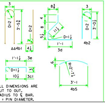
ALL DIMENSIONS ARE OUT TO OUT. RADIUS TO C. BAR. D = PIN DIAMETER.
