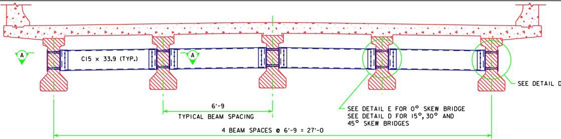
SECTION SHOWING INTERMEDIATE DIAPHRAGM
