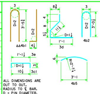
ALL DIMENSIONS ARE OUT TO OUT. RADIUS TO @ BAR. D = PIN DIAMETER.
