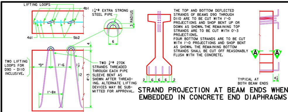
**STRAND PROJECTION AT BEAM ENDS WHEN EMBEDDED IN CONCRETE END DIAPHRAGMS**
