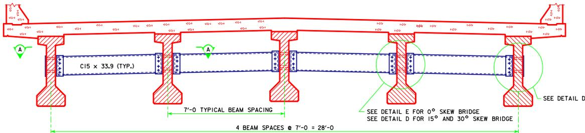
SECTION SHOWING INTERMEDIATE DIAPHRAGM
