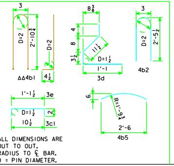
ALL DIMENSIONS ARE OUT TO OUT. RADIUS TO C. BAR. D = PIN DIAMETER.
