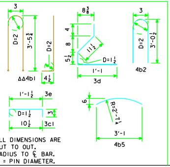
ALL DIMENSIONS ARE OUT TO OUT. RADIUS TO  $\frac{1}{2}$  BAR. D = PIN DIAMETER.
