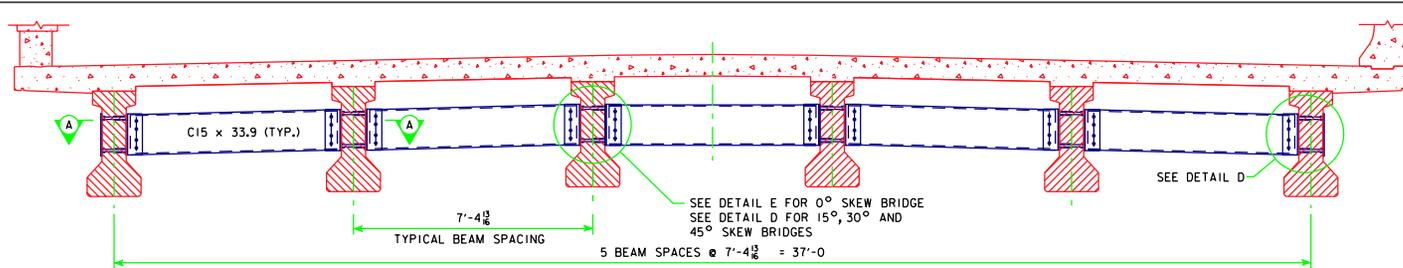
SECTION SHOWING INTERMEDIATE DIAPHRAGM
