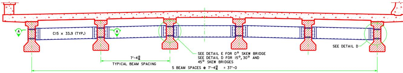
SECTION SHOWING INTERMEDIATE DIAPHRAGM
