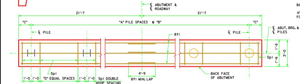
**ABUTMENT PILE PLAN**
