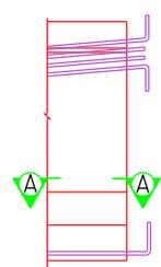
STRAND PROJECTION AT BEAM ENDS WHEN EMBEDDED IN CONCRETE END DIAPHRAGMS
