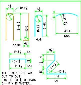
ALL DIMENSIONS ARE OUT TO OUT. RADIUS TO C OF BAR. D = PIN DIAMETER.
