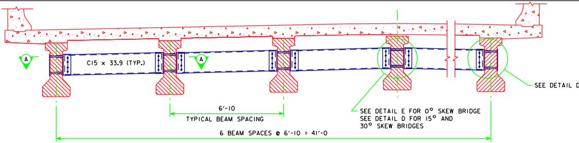
SECTION SHOWING INTERMEDIATE DIAPHRAGM
