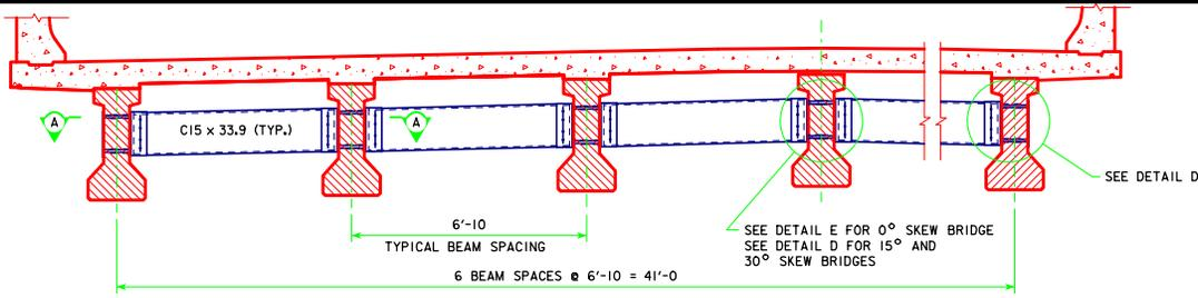
SECTION SHOWING INTERMEDIATE DIAPHRAGM
