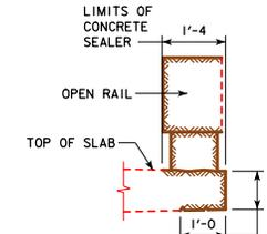
**CONCRETE SEALER LIMITS FOR OPEN RAILS**
