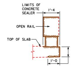
**CONCRETE SEALER LIMITS FOR OPEN RAILS**
