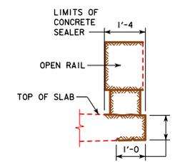
**CONCRETE SEALER LIMITS FOR OPEN RAILS**
