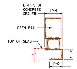
**CONCRETE SEALER LIMITS FOR OPEN RAILS**
