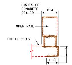
**CONCRETE SEALER LIMITS FOR OPEN RAILS**
