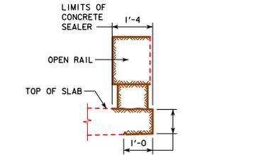
**CONCRETE SEALER LIMITS FOR OPEN RAILS**
