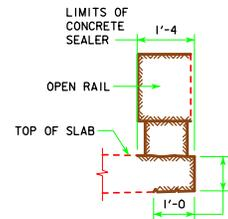
**CONCRETE SEALER LIMITS FOR OPEN RAILS**
