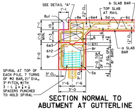
SECTION NORMAL TO ABUTMENT AT GUTTERLINE
