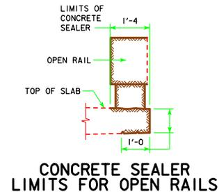
**CONCRETE SEALER LIMITS FOR OPEN RAILS**
