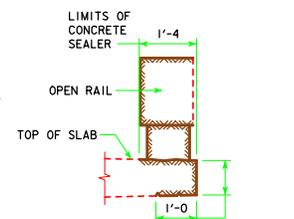
**CONCRETE SEALER LIMITS FOR OPEN RAILS**
