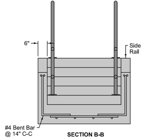
Provide a minimum of 2 inches of cover for all reinforcing.
